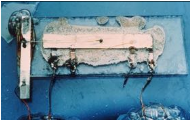
1958 - First integrated circuit, Jack Kilby
