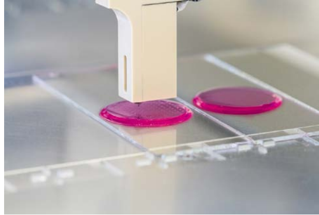
Figure 4.2. An inkjet printer developed by Fraunhofer IGB scientists for printing cell suspensions onto shimmering pink hydrogel pads, which prevent desiccation (courtesy of and © Fraunhofer IGB).
