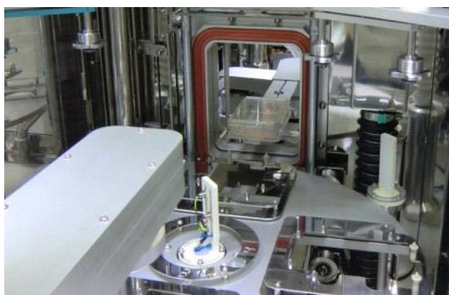
Figure 4.5. Cell sheet factory-automated cell culture system (courtesy of Prof. Teruo Okano).
