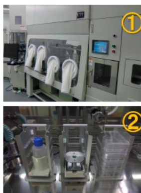
Figure 6.3. T-Factory, an automation system for cell-sheet biomanufacturing (courtesy of Tokyo Women's Medical University).
