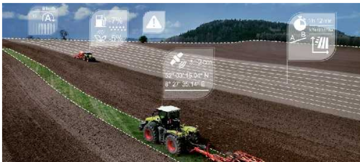
Figure 10. Use of GPS leads to reduction in fuel consumption and improved timeliness of operations
