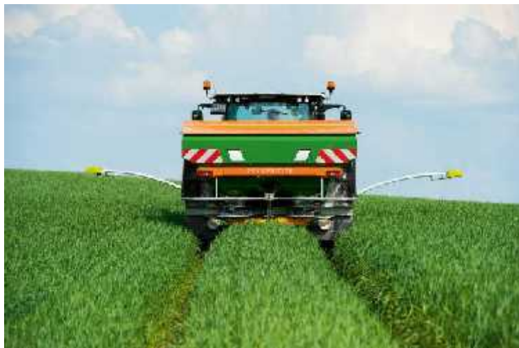
Figure 4. Sensing of crop Nitrogen stress for precision fertilizer application
