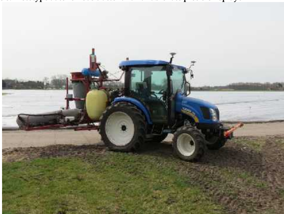
Figure 8. Prototype autonomous tractor and variable rate precision sprayer
