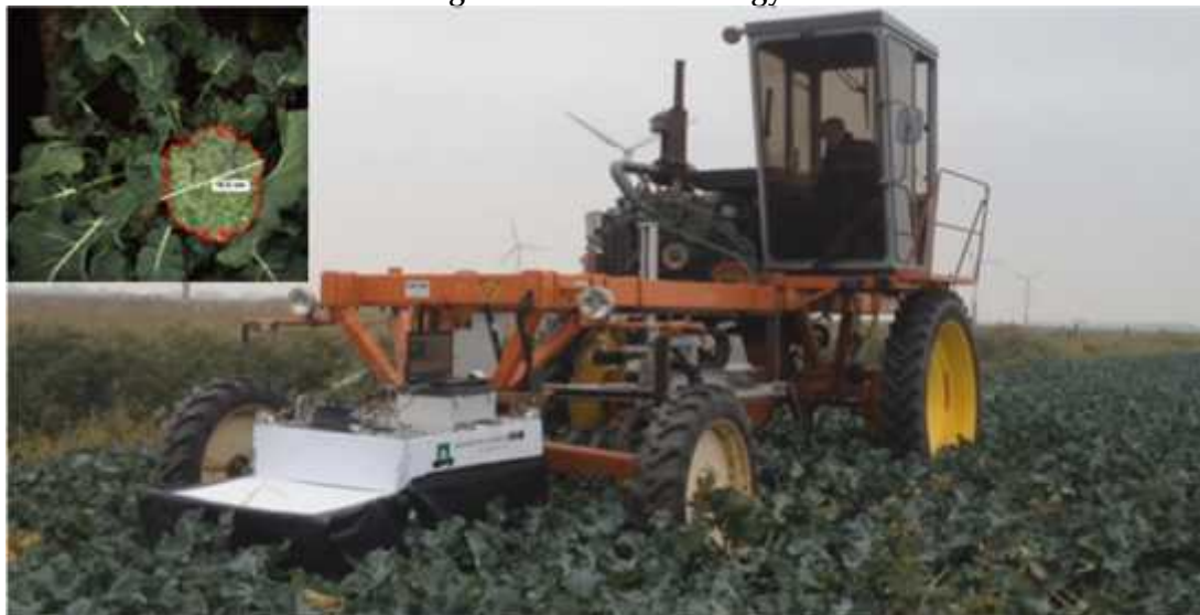
Figure 12. Selective broccoli harvesting with sensor technology on harvester
