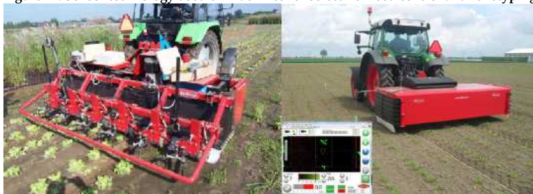
Figure 11. Sensor technology used on machines for selective weed control and fenotyping
