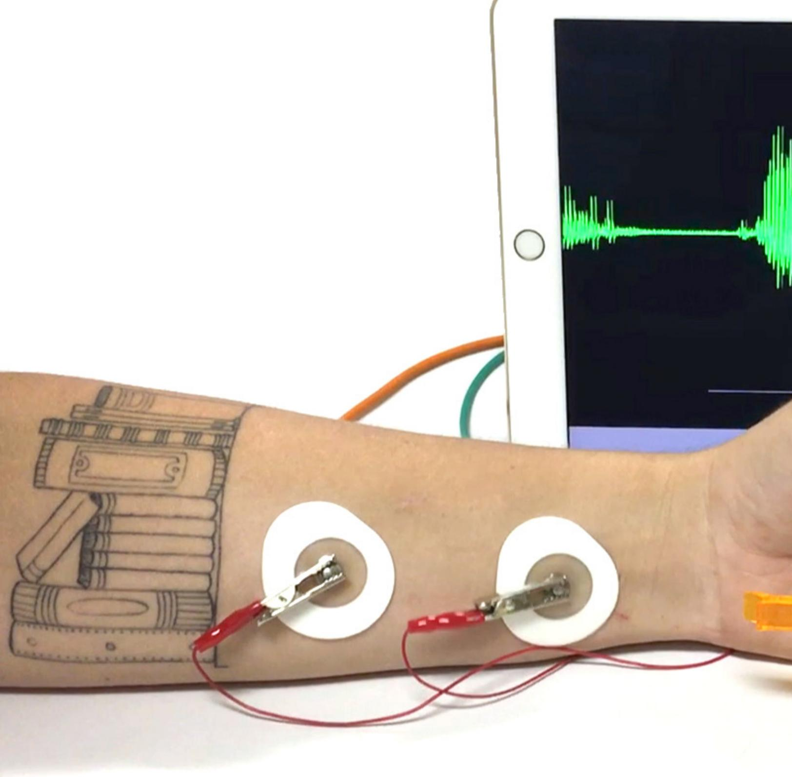
The Claw: An open-source neuroprosthetic for education that turns electromyography into servo action to close (a) and open (b) a claw device. Backyard Brains, CC-BY-SA, 2016
