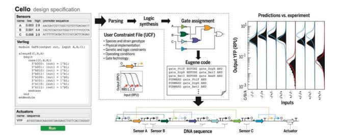
**FIGURE 4-3** Illustration of genetic circuit engineering facilitated by a software environment that couples circuit specification and design to predictive models of circuit function. NOTE: Genetic circuits are a common staple for work in synthetic biology and allow users to combine multiple functions from the broad categories of sense, compute, and actuate. SOURCE: Nielsen et al., 2016.
