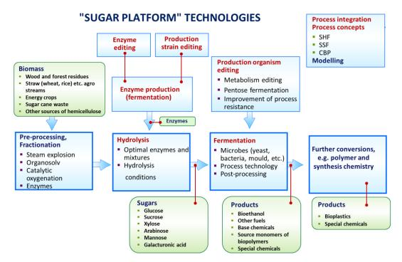
Fermentation of biomass sugars into different fuels and chemicals using genetically engineered microbes is one of the most important production concepts of bioeconomy.
