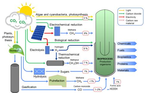
Proposal on the possible routes for carbon dioxide (CO<sub>2</sub>) conversion into carbon sources suitable for bioprocesses. The percentages indicate the energy efficiency of the conversion in accordance with the first law of thermodynamics (light, electricity and chemical energy were treated equally). The photosynthesis of algae and cyanobacteria produces biomass that may also already contain the desired product. Image: Juha-Pekka Pitkänen & Peter Blomberg
