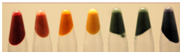
Color output of the Cambridge team's biosensor part.
